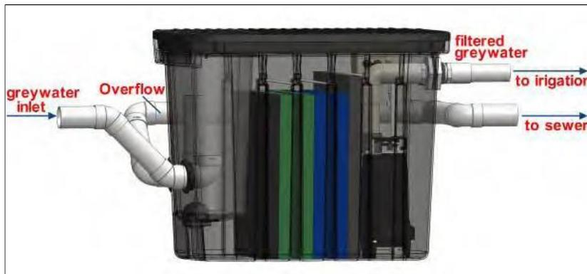
To create the overflow to sewage, at the inside of the basket, add on a short piece of pipe to the upside turned elbow. Once installed the top of this pipe should be at the same level as the top of the installed black sheet.
